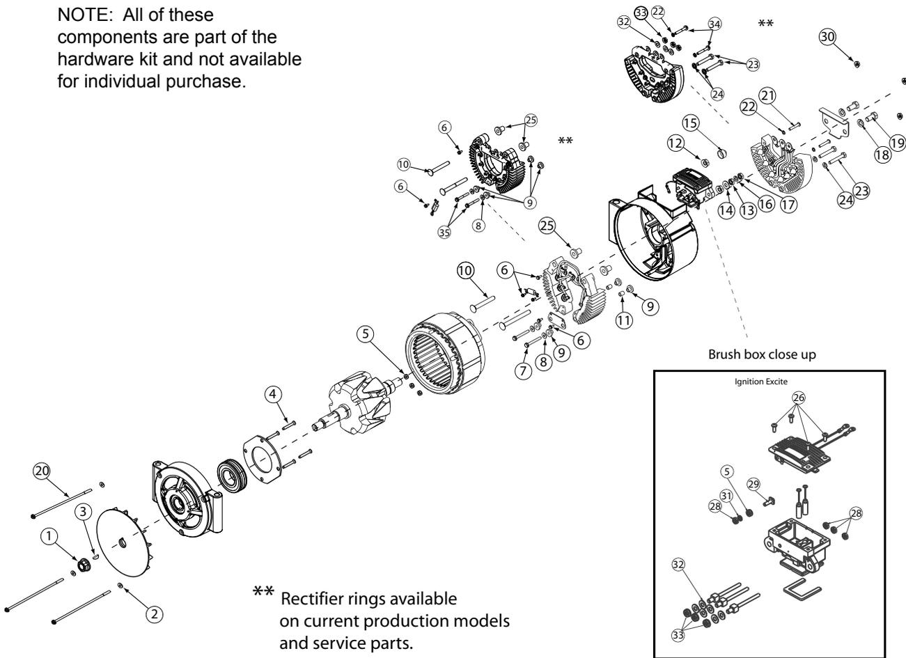
\*\* Rectifier rings available on current production models and service parts.
